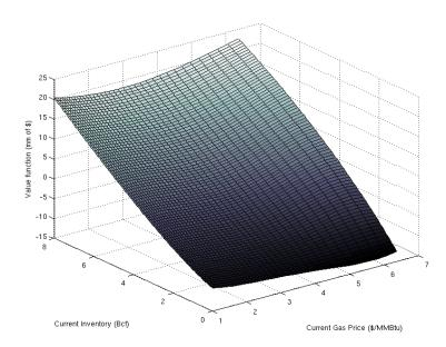
Figure 1 Value function surface for Example 1 showing V(0.5, g, c, store; T = 1) as a function of current gas price  $G_t = g$  and current inventory  $C_t = c$ .
